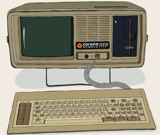
The PPC-400 Corona microcomputer, the first portable model used by field examiners, weighed 28 pounds and had a 10MB hard drive and 512MB of memory
